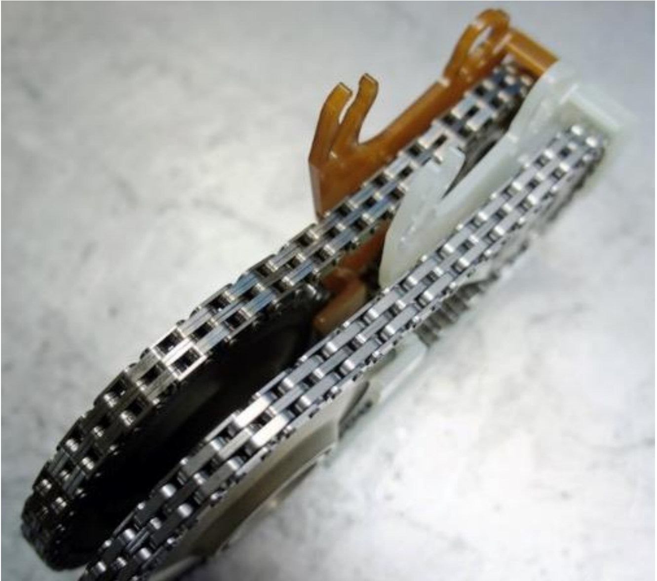
FIGURE 4: ORIGINAL AND REVISED CLASS ENGINE OIL PUMP CHAIN DRIVE 9
